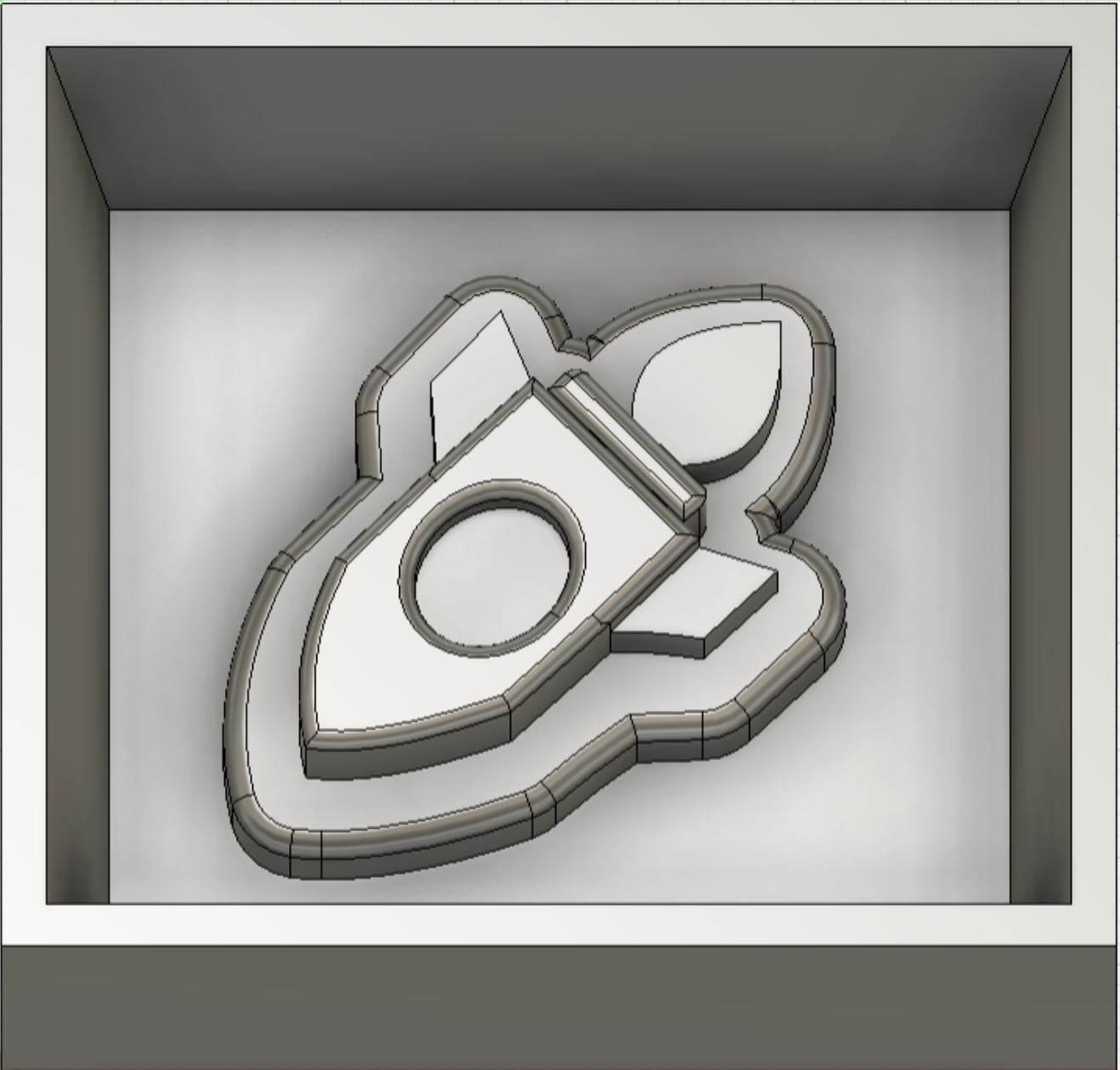
In the Manufacturing workbench we create a setup, with a stock of 0-offset and the origin bottom-left at the upper corner:
