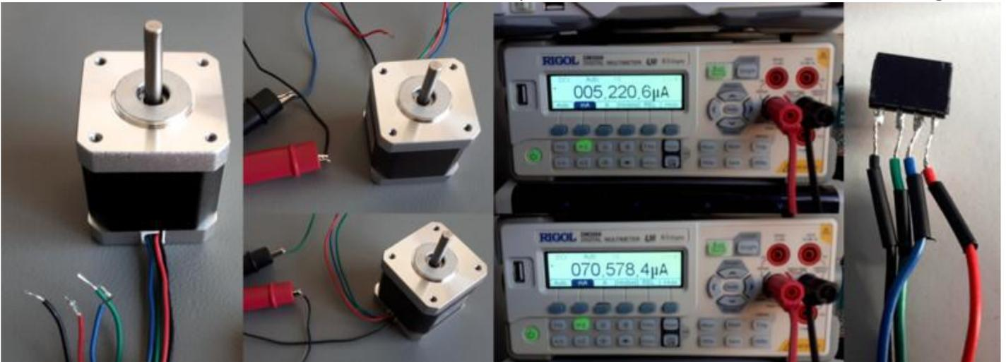
We soldered the cables so that the corresponding cables were next to each other. The next question was: does the motor turn the right way around? The direction of the motor could be changed without changing the firmware by just switching the cables. The following rules hold where `1A 1B 2A 2B` is the original order of the cables:
