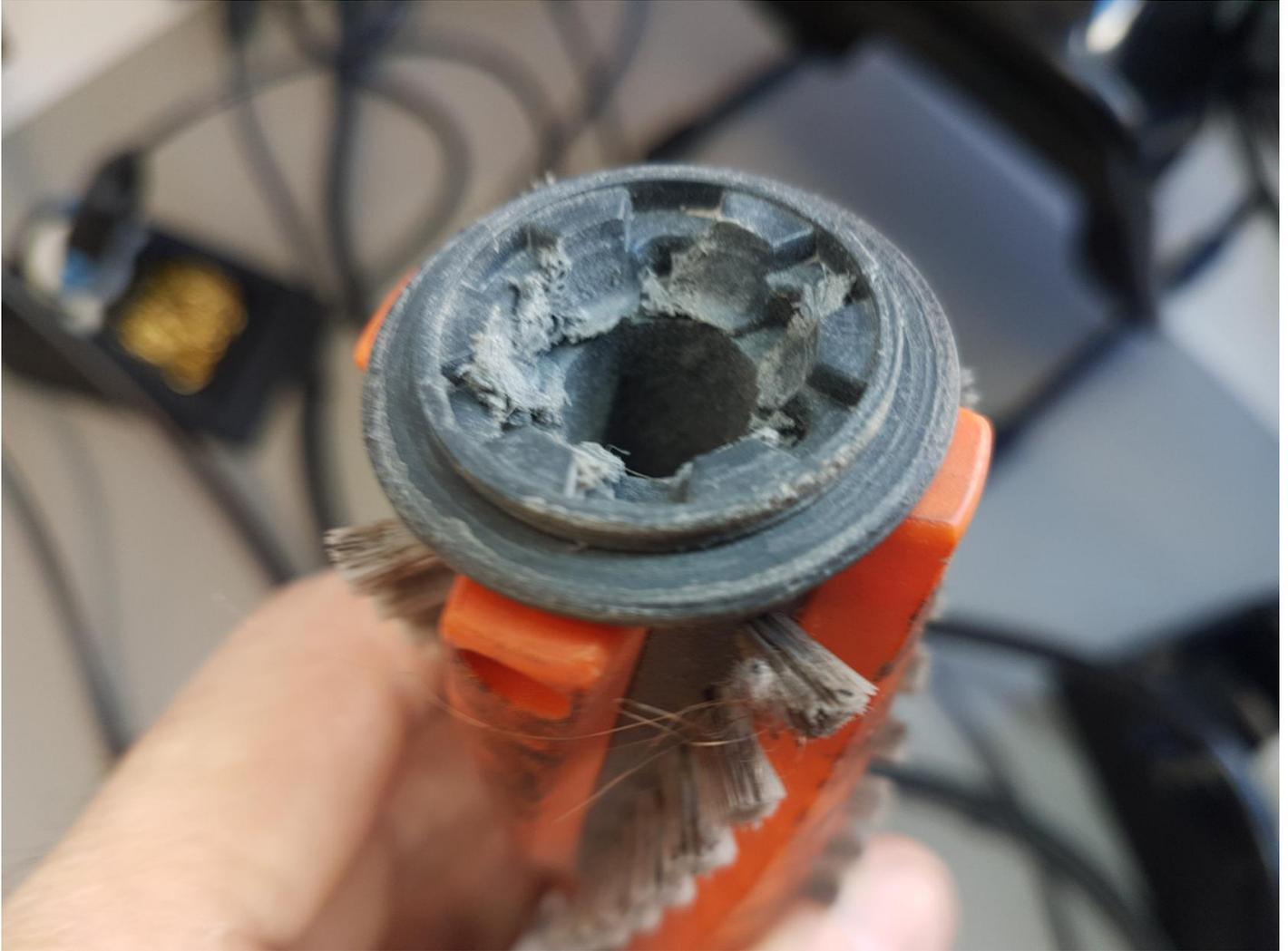
I 3D-scanned the clutch with our CR-Scan Raptor in blue laser mode. For this to work, you need several tracking points around the object.
