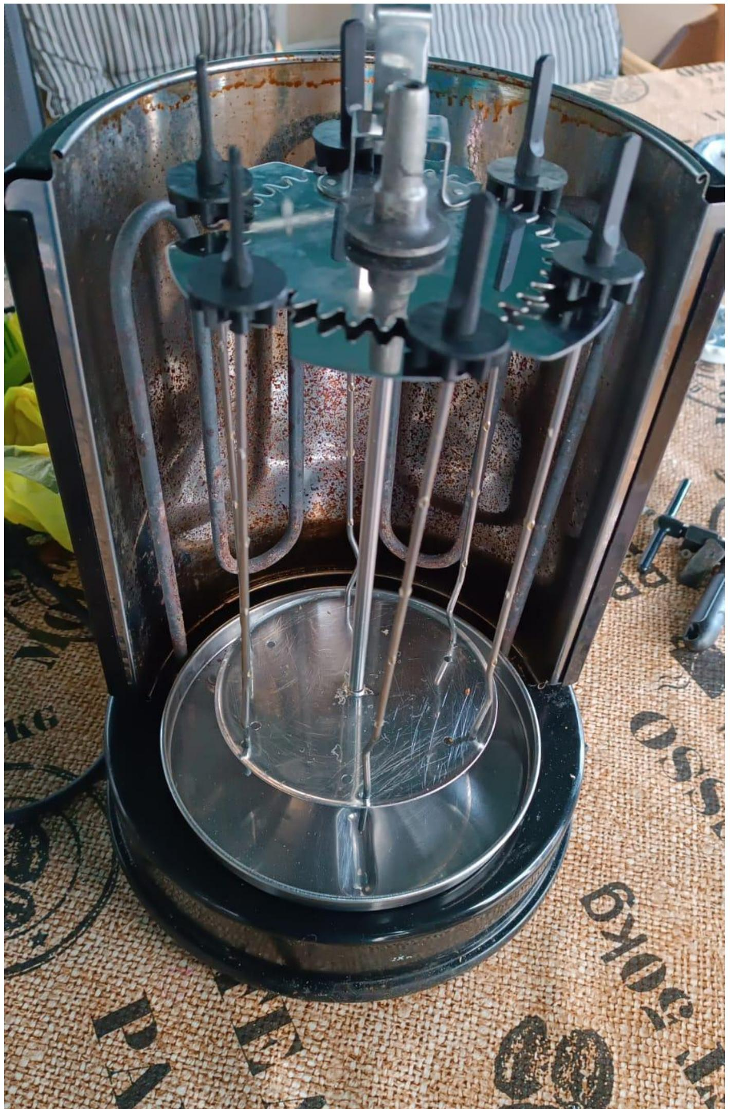
The most difficult part was getting the gear right. I measured the inner and outer diameter of the gear (Kopfkreis Ø 25 mm and Fußkreis Ø 14 mm) and then asked DeepSeek for the modulus of the gear. The first time I didn't give it the amount of teeth and it gave me a long but useless answer. The second time it told me that the module is 2,5. Which turns out to be perfectly right. I used the Gear-Module in FreeCAD to model this gear:
